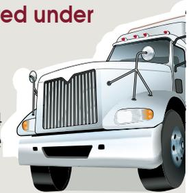
The *gross vehicle weight rating*, which is determined by the manufacturer, represents **the weight of the vehicle, plus the maximum load the vehicle can carry.**
