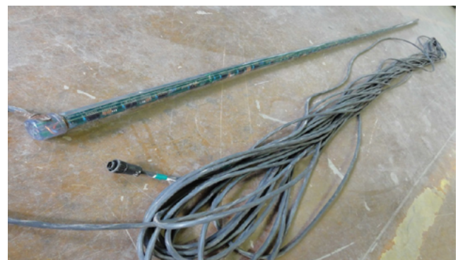
Figure 3: Electronic frost depth probe
