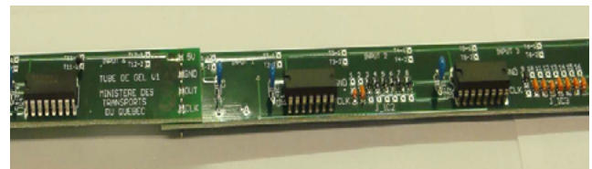
Figure 2: Overview of printed circuits of the electronic frost depth probe
