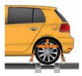
Tiedowns that are designed to attach to the structure of a light vehicle must be attached to the mounting points on the vehicle that are specifically designed for that purpose.
