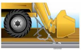
The accessory equipment on a heavy vehicle (e.g. hydraulic shovels) must be completely lowered and secured to the vehicle, unless the equipment:
