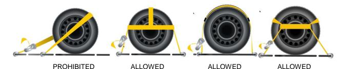
In cases where tie-downs are installed on wheels in a way that could make the vehicle rotate because they produce tension only toward the front and the rear (without being centered with the longitudinal central axis—Illustration 1), it is mandatory to install a tie down at each of the four corners of the vehicle to prevent any possibility of rotation (which would loosen tie-downs). The same applies to tie-downs that produce lateral tension on a front wheel and a rear wheel (Illustration 2).
