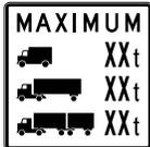
Weight restrictions for various types of trucks authorized to cross a bridge according to the number of units. This sign is installed near bridges and overpasses. It also applies to bus drivers.
