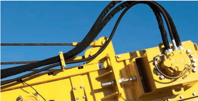
**Direct Drive Motors with Loop Flushing**
