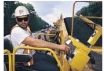
The main control console, located at the left side control station, serves as the main electrical junction box. Additionally, operator control/reference for left/right console selector switch, tachometer/hour meter, parking brake warning light and analog gauges for engine oil pressure, coolant temperature, hydraulic oil temperature and voltmeter are located on this main console. On-off control of the optional generator set is also included if the unit is so equipped.
