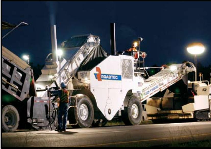
The SB-1500D Shuttle Buggy® material transfer vehicle features a low weight and a narrow transport width. It can store up to 15 tons (13.6 MT) of asphalt mix, allowing haul vehicles to unload as soon as they arrive. This substantially reduces trucking costs. The SB-1500D features an end-dump hopper or an optional windrow pickup head. It also features the patented antisegregation auger which remixes materials for aggregate and temperature segregation.
