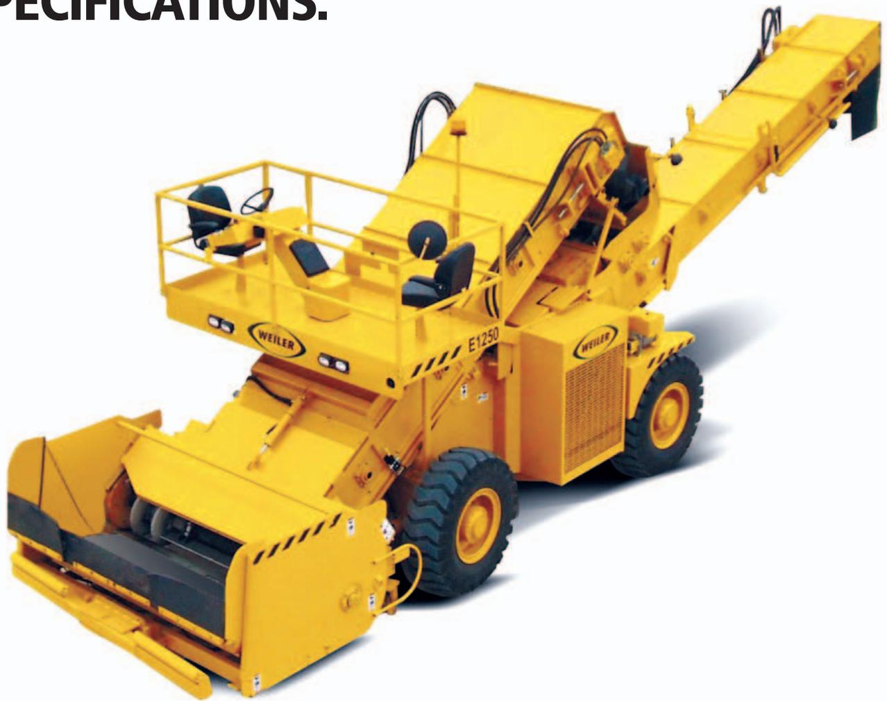
The E1250 allows for non-contact non-stop paving. The operator is given even more surge capacity by adding the optional hopper insert for the paver. The optional power remix transition hopper remixes both size and temperature segregated particles to help achieve those all important smoothness bonuses. This unit is also very versatile allowing for offset paving over barriers, string lines or any obstacle that makes it difficult to get trucks in front of the paver for inline paving.
