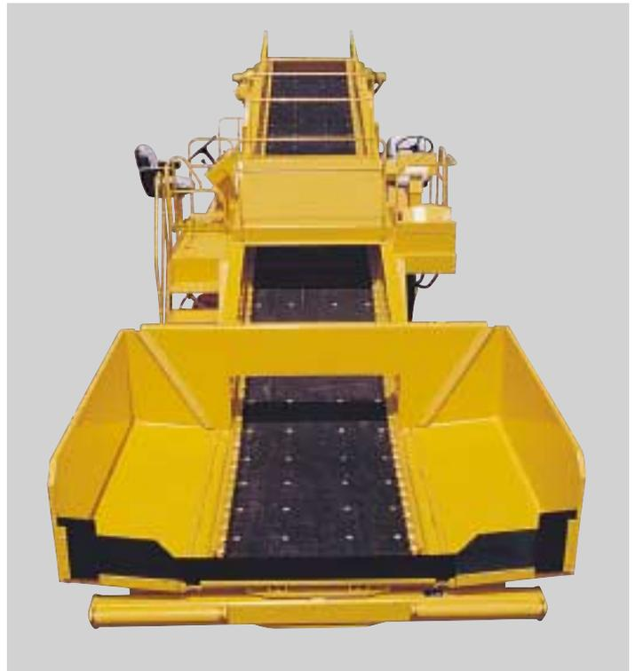
Reversible flashing, along both sides of the conveyor belt, retards material migration into the chain channels and interior conveyor structure. Chain scraper plates minimize the effect of any material migration into the chain channels by continually dragging and expelling this material out the clean-out slots located above the fines collection hopper. Two easily removable trays,
