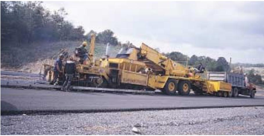
**Suspension:** The MC-330 is an extremely stable machine with a low center of gravity and excellent flotation. The long wheelbase on eight tires plus the unique front suspension geometry prevent load concentration that could displace base material or break through old surface materials.
