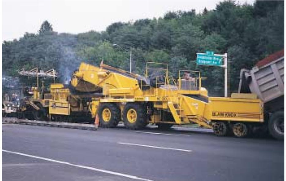
Width—Overall (hopper sides up) . . . . . 10'1<sup>3</sup>/<sub>8</sub>" (3.08 m)
