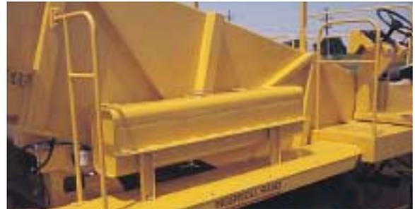
Both the Main and Optional Swing Conveyors are equipped with a belt spray system for spraying of any fluid (biodegradable recommended) onto the belt(s) to help prevent asphalt build-up. The system incorporates a series of filtered spray nozzles, pump, electric switch control(s), and a 40 gal. (151.4 L) reservoir tank with replaceable filter.
