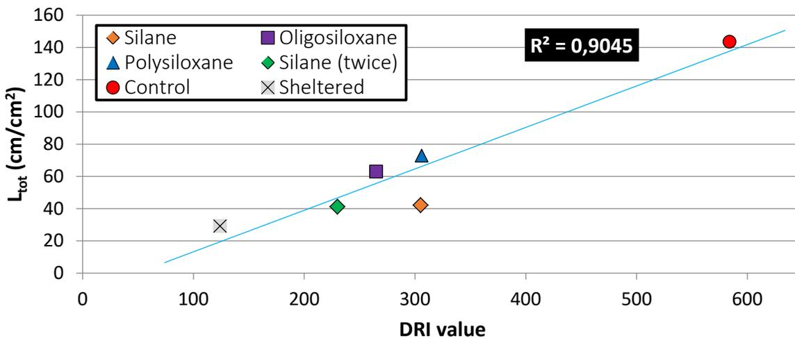
Figure 4: Comparison of the crack mapping in the form of total length of cracking determined by image analysis and the internal damage determined by DRI.
