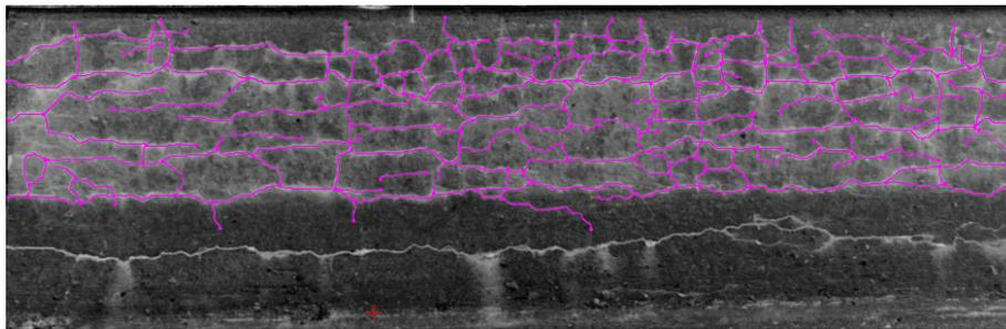
Figure 1: Example of crack tracing using the Simple Neurite Tracer plugin in ImageJ.
