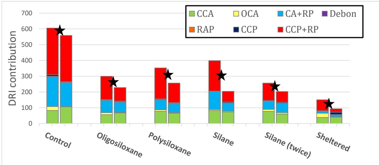
Figure 3: Internal damage assessment of all cores (two per section) displayed as DRI bar charts showing the contribution of each petrographic features; the black star indicates the average DRI values for each set of cores from the different barrier sections. The acronyms are defined in Table 1.
