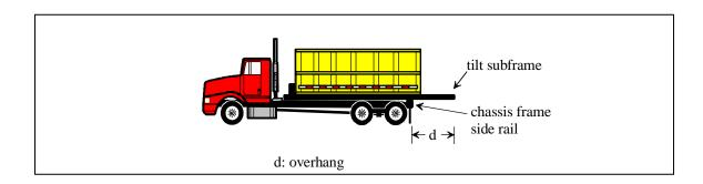
When the overhang is one metre or less, there are no special requirements. This is the case of certain telescopic roll-on roll-offs. However, when the rear end of the load or equipment extends beyond the end of the vehicle by more than one metre at its farthest point, section 474 du *Highway Safety Code* prescribes the installation of a red flag or a reflector panel during the day, and, at night, a red light visible from behind and from the sides for not less than 150 metres.
