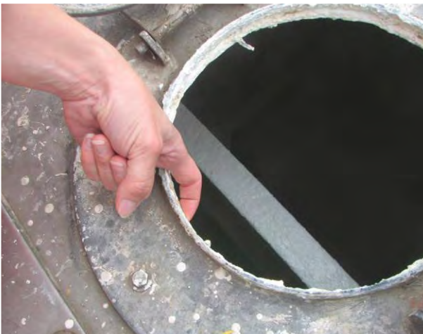
Figure 22 – Example of reference point for taking measurements
