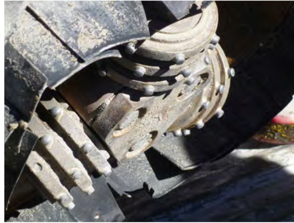
Figure 67 – Blades on the bottom of a hand removal unit
