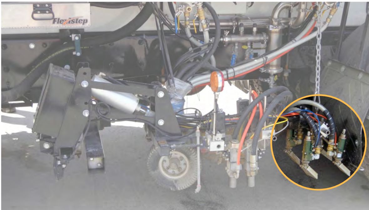
Figure 45 – Example of glass microbead applicator guns
