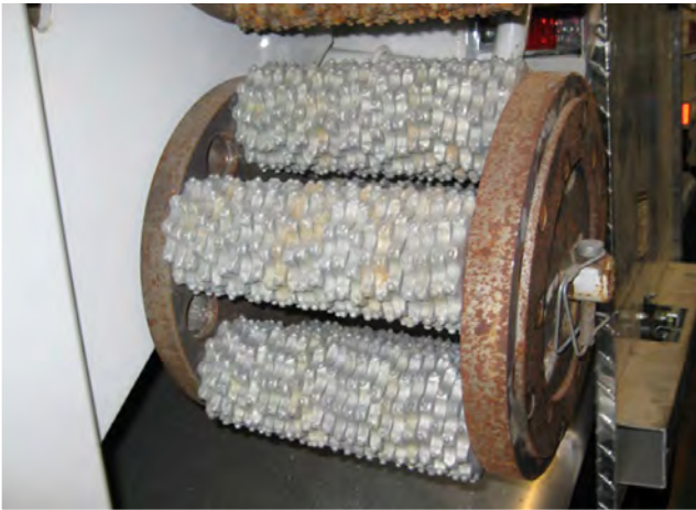
Figure 65 – Blade assembly for removal by mechanical abrasion
