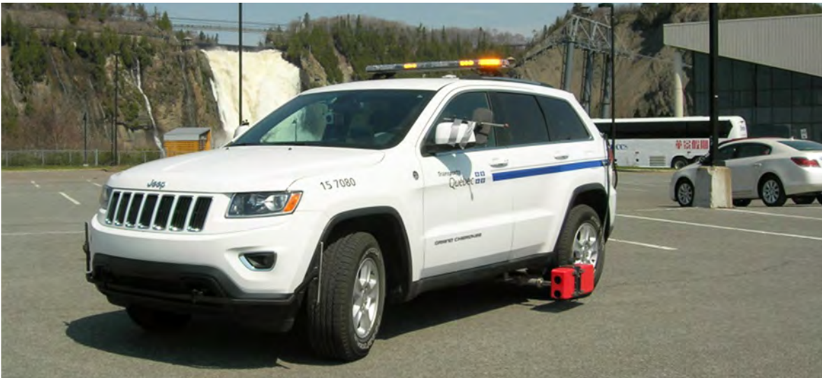
Figure 51 – Vehicle-mounted mobile retroreflectometer
