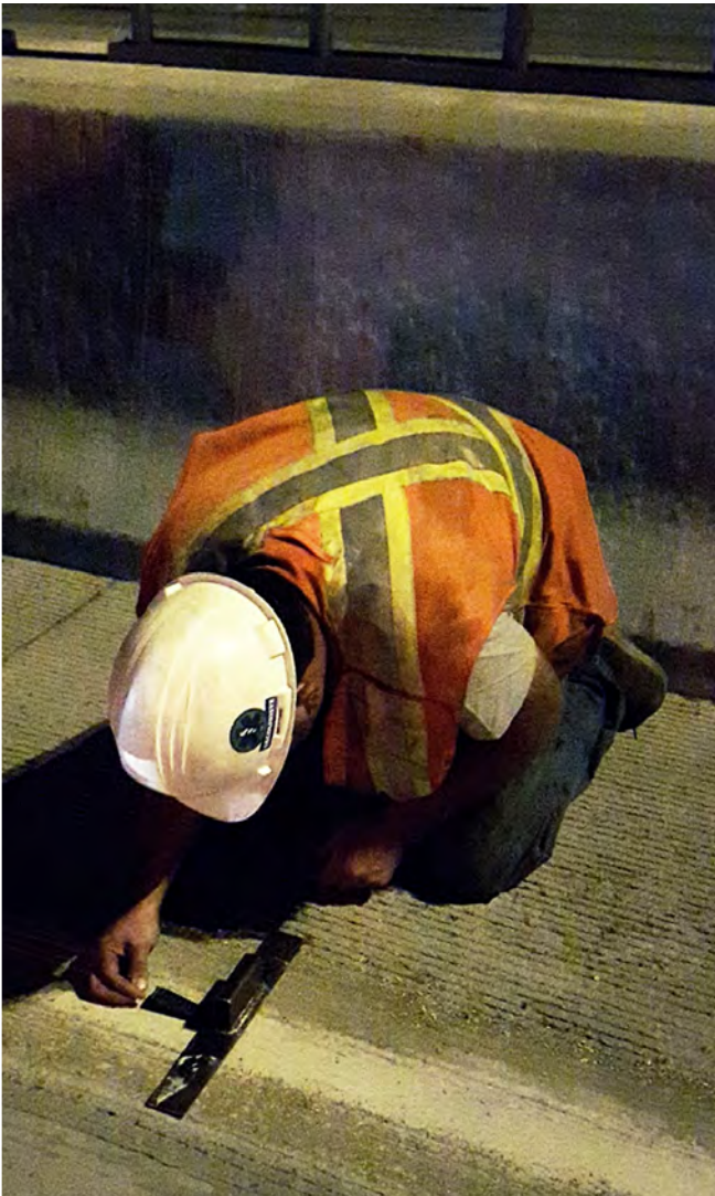
Figure 36 – Example of measuring with a conical gauge
