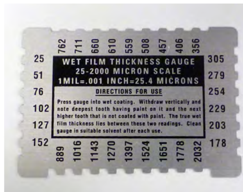
Figure 25 – Thickness gauge ( \mu\text{m} )
