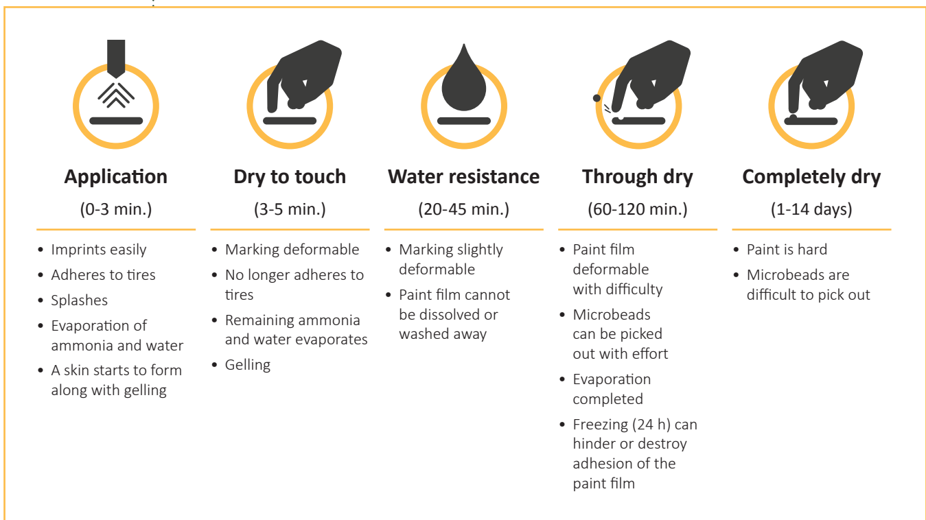
Figure 15 – Stages of how water-based pavement marking paint dries
