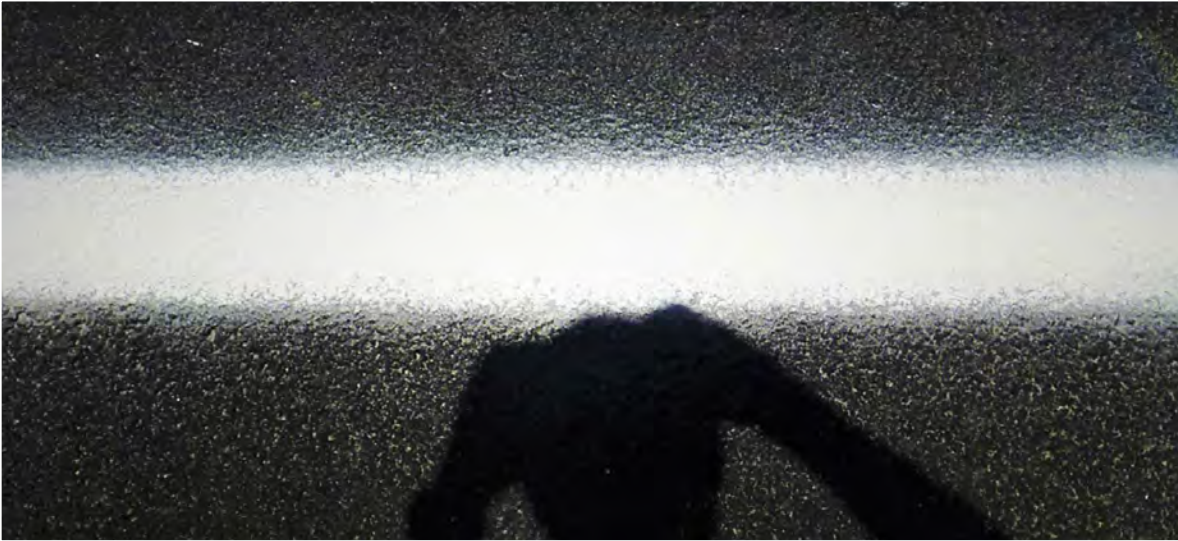
Figure 48 – Example of adequate dispersion of glass microbeads
