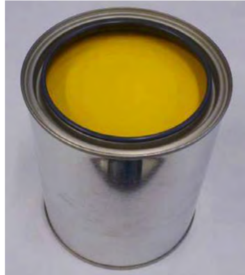
Figure 19 – Example of container properly filled
