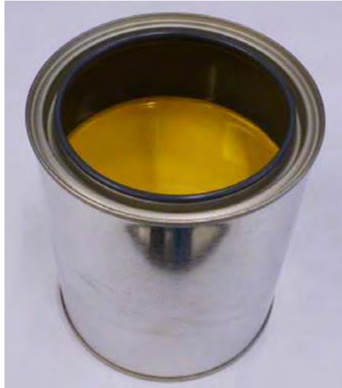
Figure 18 – Example of container insufficiently filled
