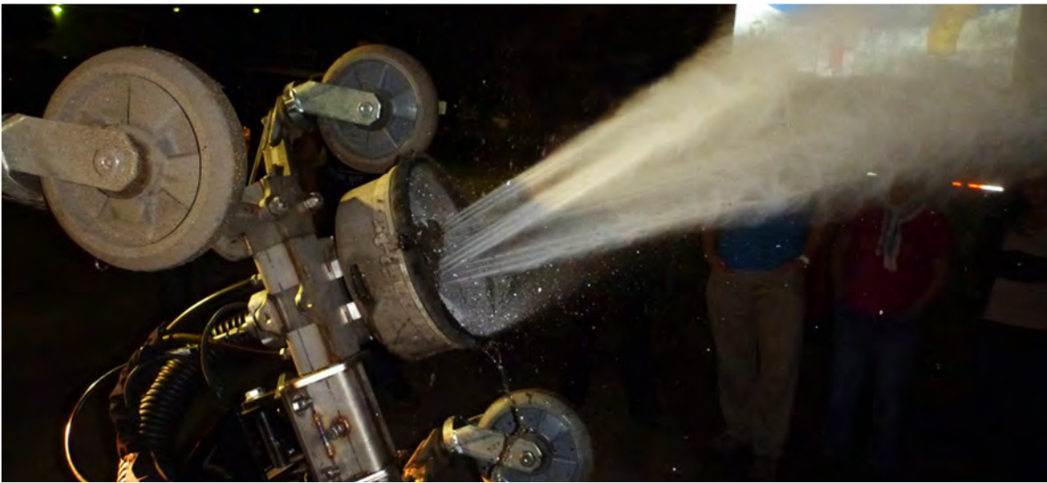
Figure 70 – High-pressure water blasting
