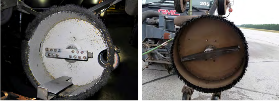
Figure 71 – Heads with high-pressure water jets
