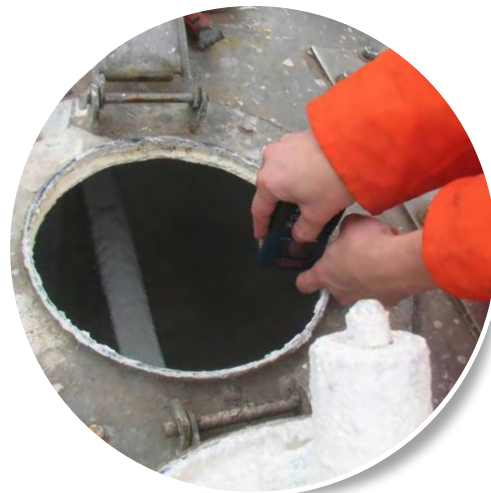
Figure 23 – Taking measurements, using the reference point
