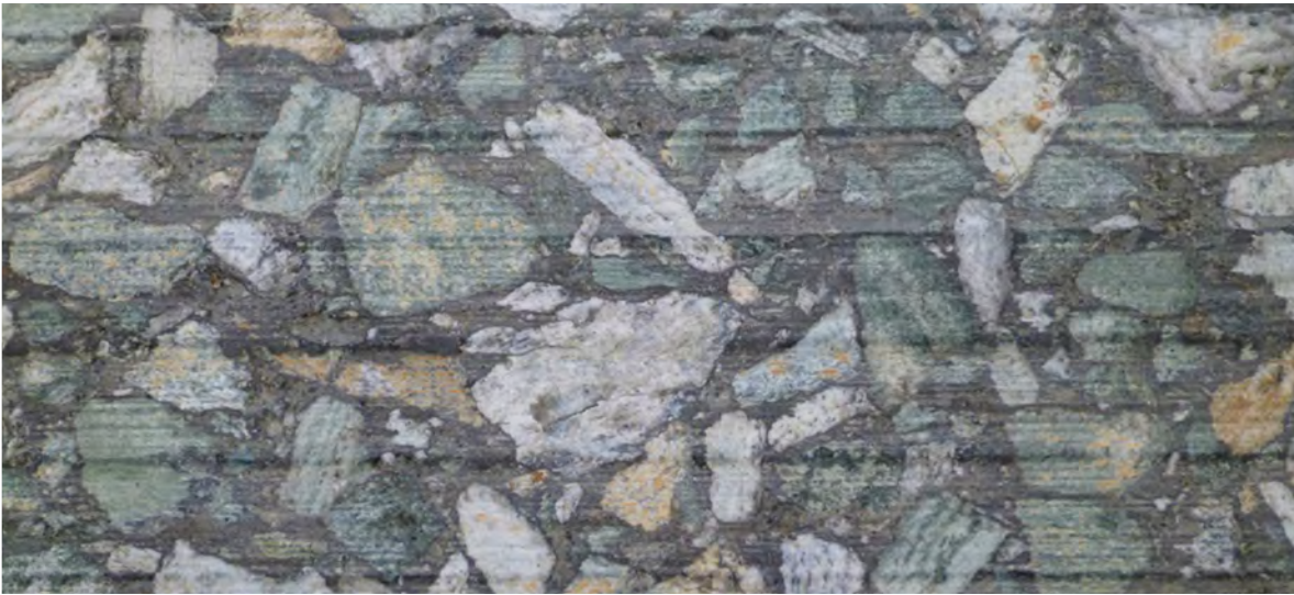
Figure 32 – Example of compliant smooth-finish groove (close-up)
