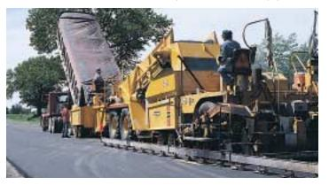
**Suspension:** The MC-330 is an extremely stable machine with a low center of gravity and excellent flotation. The long wheelbase on eight tires plus the unique front suspension geometry prevent load concentration that could displace base material or break through old surface materials.
