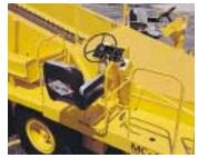
**Brakes:** Primary braking is accomplished through the dynamics of the hydrostatic traction drive system. Foot actuated, hydraulic caliper/disc secondary brakes, mounted on the output ends of the axle, provide secondary/back-up brake control. An independent, spring applied parking brake is automatically actuated when the ignition switch is turned off or electrical power is lost. The parking brake can also be manually applied via an electrical switch on either operator's control console.
