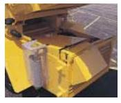
located under the main conveyor, shield the engine and drive componentry from any material carry-back, and provide for quick, easy clean-out of any material accumulation.
