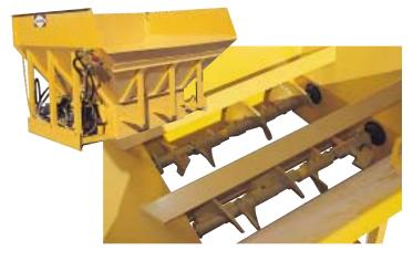
**Twin Auger Remixing Tub:** 14 ton (12.7 T) paver hopper insert with two transverse mixing augers. Functioning in opposing directions, the augers create a vortical flow in the paving material to re-mix and blend the entire material volume to a more homogeneous consistency; virtually eliminates material segregation. Unit is hydraulically powered from either the MC-330 or the paver.
