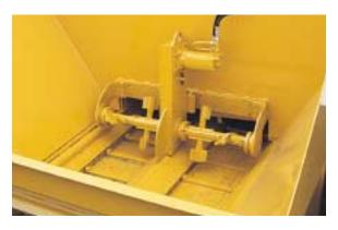
**Mixer/Agitator:** A patented, self-contained, mixing/blending unit mounted in the Optional Hopper Insert. With paddles counterrotating relative to the paver's feed conveyors direction of travel, the unit remixes the paving material to minimize end-of-load segregation. Unit is powered hydraulically from either the MC-330 or the paver.
