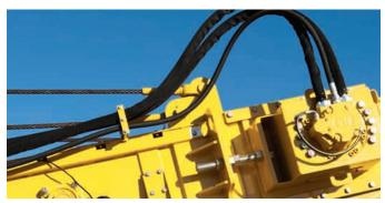
Direct Drive Motors with Loop Flushing
