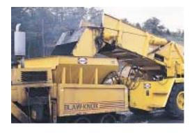
**Hopper Insert:** 20 ton (18.1 T) [315 cubic feet (8.92 m³) struck] capacity; fits into the existing hopper of the paver performing the laydown operation to further increase material surge storage capacity for quicker, more efficient truck unloading and a smoother, uninterrupted laydown operation.
