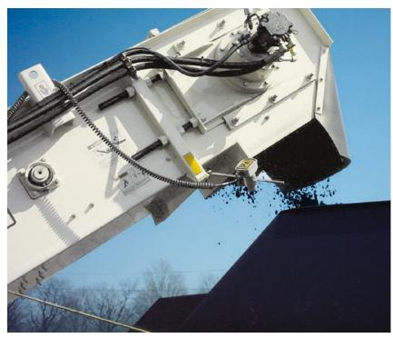
Rugged high-capacity conveyors reduce chance of asphalt temperature loss
