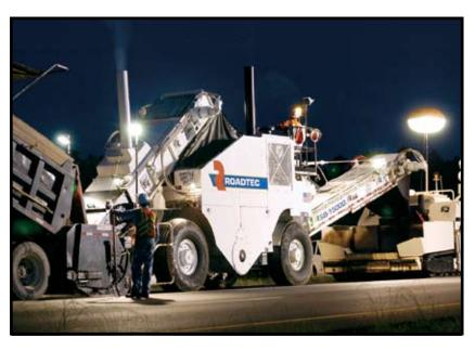
The SB-1500D Shuttle Buggy® material transfer vehicle features a low weight and a narrow transport width. It can store up to 15 tons (13.6 MT) of asphalt mix, allowing haul vehicles to unload as soon as they arrive. This substantially reduces trucking costs. The SB-1500D features an end-dump hopper or an optional windrow pickup head. It also features the patented antisegregation auger which remixes materials for aggregate and temperature segregation.
