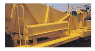
Both the Main and Optional Swing Conveyors are equipped with a belt spray system for spraying of any fluid (biodegradable recommended) onto the belt(s) to help prevent asphalt build-up. The system incorporates a series of filtered spray nozzles, pump, electric switch control(s), and a 40 gal. (151.4 L) reservoir tank with replaceable filter.
