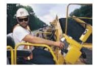
and 2-speed axle; main conveyor function, speed, direction and spray bar; foldinghopper, horn and parking brake. Electric switch controls for the optional swing conveyor and truck hitch are also included if the unit is so equipped.
