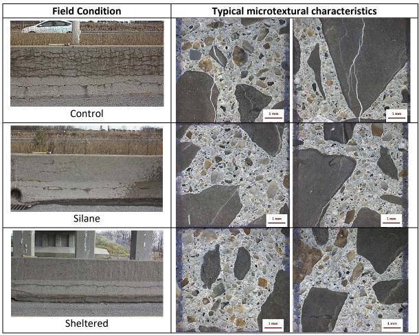
Figure 2: Comparison of the field condition of the control, the silane treated and the sheltered barrier sections, along with typical microtextural characteristics observed at  $\approx$ 15x.
