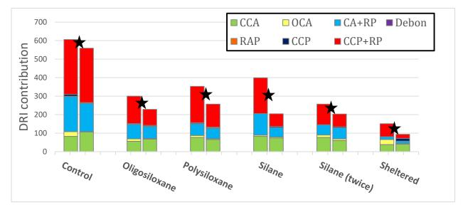
Figure 3: Internal damage assessment of all cores (two per section) displayed as DRI bar charts showing the contribution of each petrographic features; the black star indicates the average DRI values for each set of cores from the different barrier sections. The acronyms are defined in Table 1.
